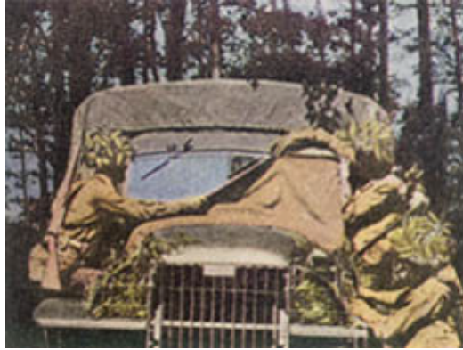
FIGURE 20. •Blankets, shelter halves, or pieces of dark coloured burlap or osnaburg are expedients for covering the reflecting surface of a windshield quickly. Foliage may be used to cover headlights.
